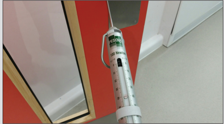
Using a Pesola Gauge to measure the opening force of a door.
